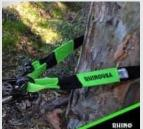
Tree Saver-A tree saver is a small strap used to wrap around a tree to prevent damage to the tree. Wrapping your winch cable around a tree can damage the tree or even kill it.
